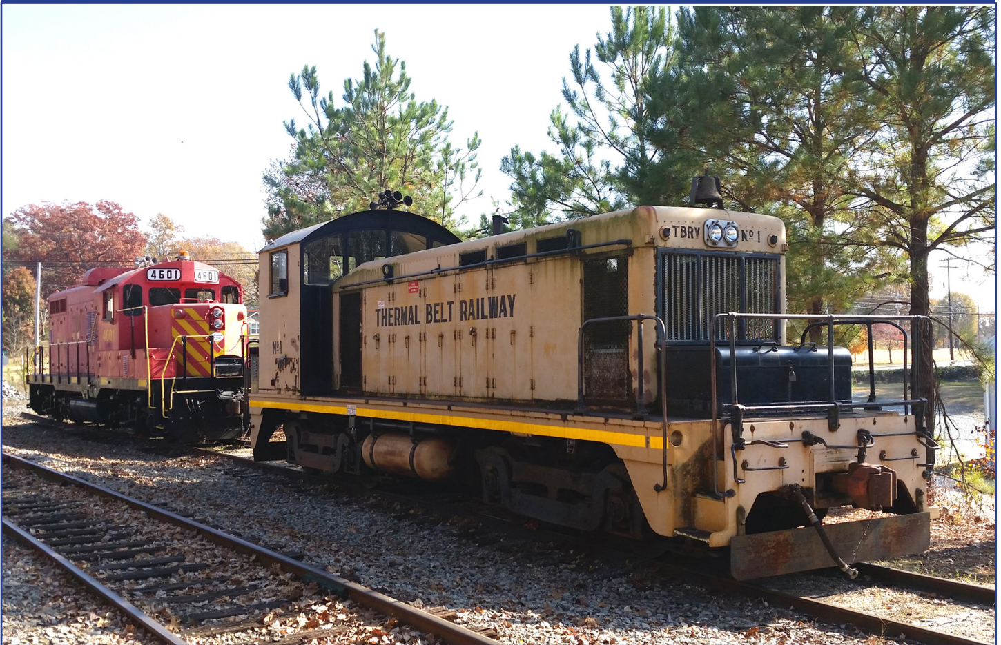
Thermal Belt Railway has added an ex-Army GP-9u (aka to some as a "GP-10") to its roster. 4601 is shown in Bostic, NC with the road's Cummins-repowered EMC SW1 switcher. # 1 was built in 1937 with a 600 hp Winton 201A diesel. All photographs in this issue by the editor
