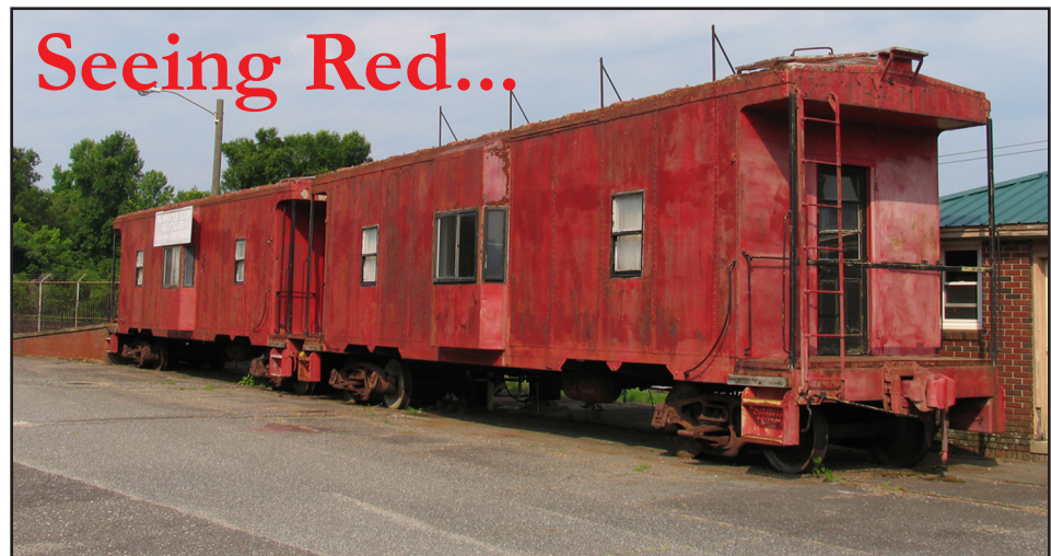
The original Norfolk Southern was a thrifty company, as seen in their box car into caboose conversions by Southern Iron and Equipment Company. NS #'s 383 (converted in 1967) and 388 (1969) are now reside next to the depot in Kings Mountain.
